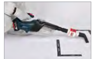
Assembled Hoover device for Total Human DNA sampling
